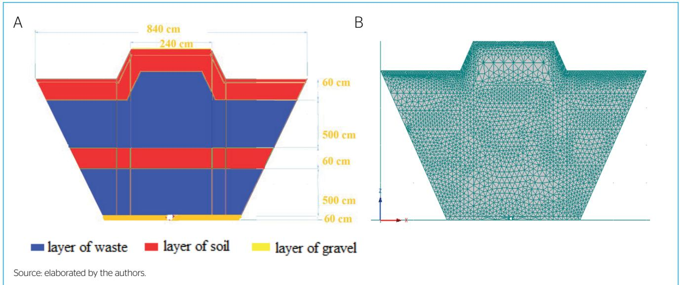
**Figure 6** - Mathematical simulation scheme: (A) geometric representation of the HYDRUS 2D numerical simulation; (B) triangular mesh used in numerical simulation.
