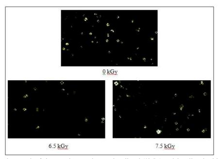
Figure 3 – Photomicrograph of rice starch granules not irradiated (0kGy) and irradiated with 6.5 kGy 7.5 kGy and observed under an optical microscope under polarized light (1000x).
