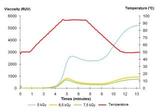
Figure 2 – Viscoelastograph profiles, measured by a Rapid Visco Analyzer (3 g ml<sup>-1</sup>), of polished white rice without irradiation (0 kGy) and with irradiation at 6.5 kGy and 7.5 kGy.
