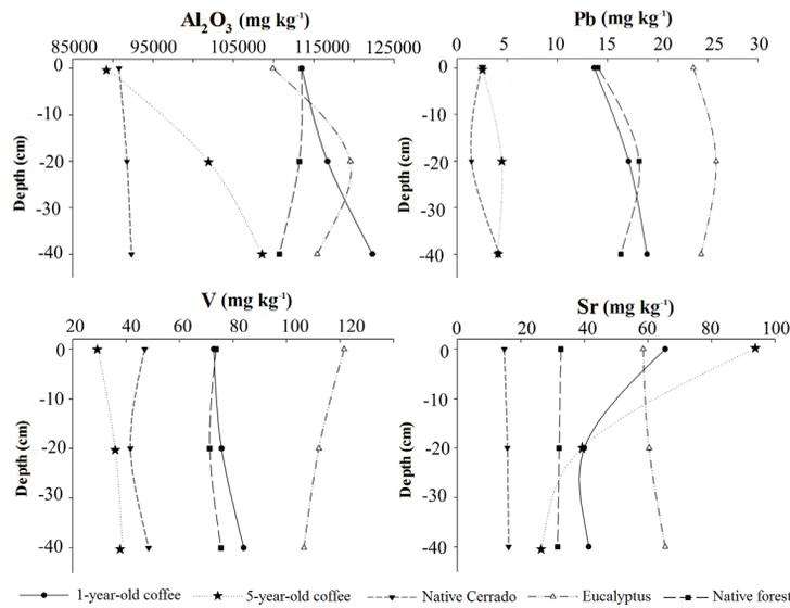
**Figure 2:** Variation of elements obtained by portable X-ray fluorescence (pXRF) spectrometry in areas with different land uses in Campos Altos, Minas Gerais, Brazil.
