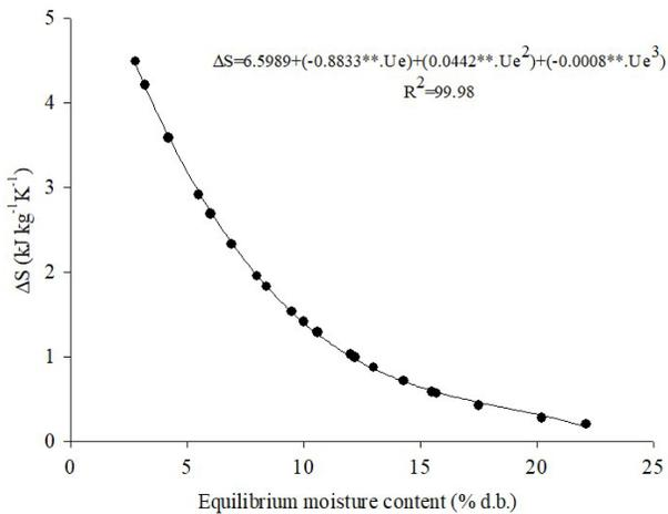
**Figure 2:** Observed and estimated values of differential ryegrass desorption entropy as a function of equilibrium moisture content.
