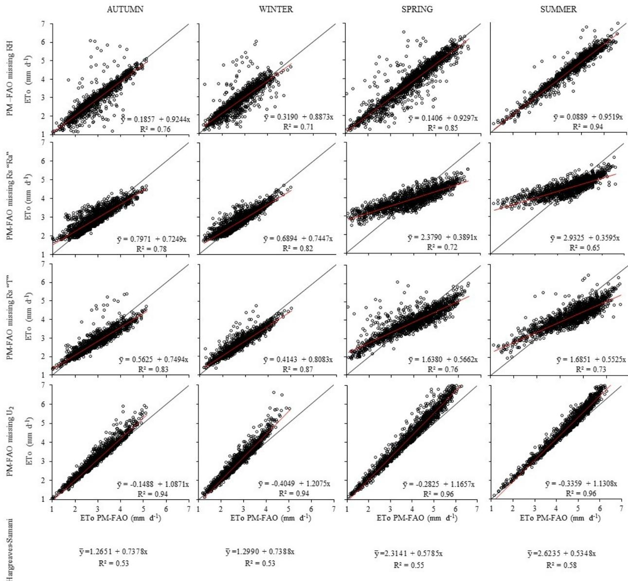
PM-FAO missing Rs "Ra" means PM-FAO with missing data of solar radiation (Rs) estimated with extraterrestrial solar radiation (Ra) and PM-FAO missing Rs "T" means PM-FAO with missing data of solar radiation (Rs) estimated with air temperature data
