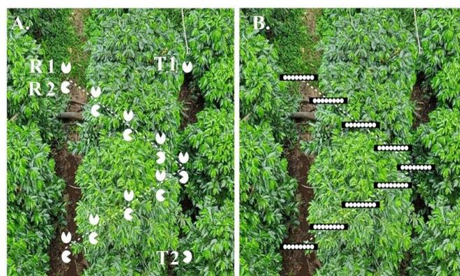
White circles show the LAI-2200C lens and the opening angle direction, parallel (T1) or perpendicular (T2) to the hedgerow. The circles marked R1 and R2 indicate the reference PAR measurements taken above the canopy. Black bars with gray circles in B indicate ceptometer bar positions at the same sampling points
