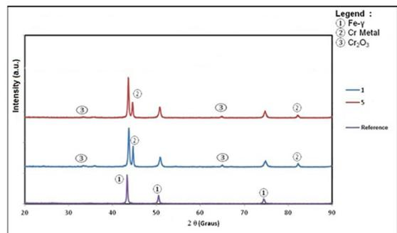
**Figure 1.** Diffractograms: of the substrate (reference) and of the samples 1 and 5.
