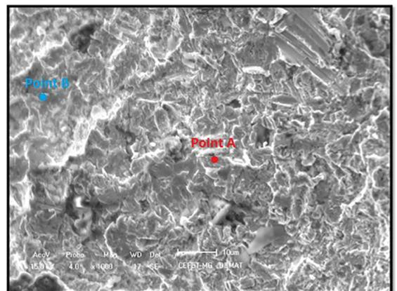
Figure 4. Microstructure of the sample 5 coated with black chromium.
