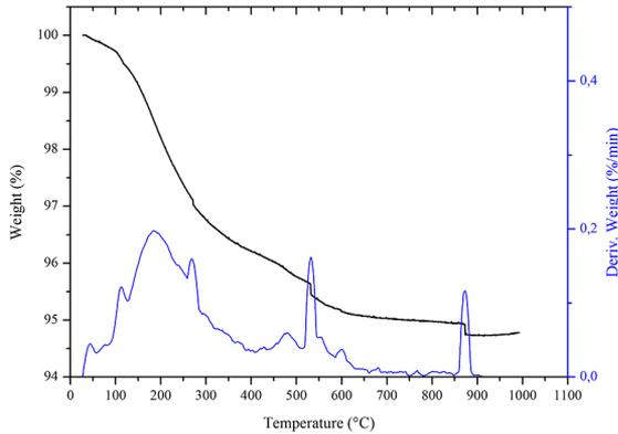
Figure 5. PExp TGA Thermal profile.
