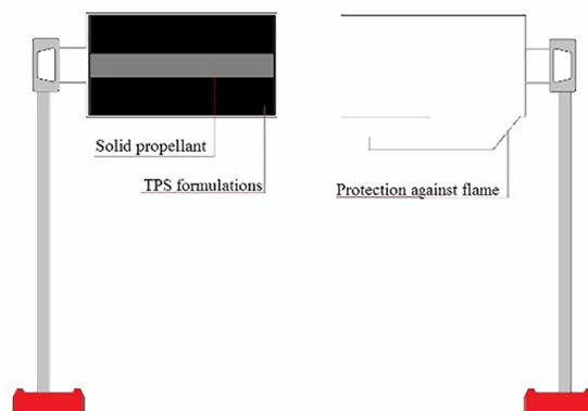
**Figure 2.** Propellant Ablation Test apparatus.
