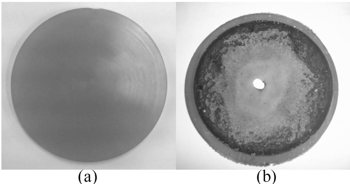
**Figure 8.** Photographs of TPS PExp-5 sample: A) before; and B) after oxy-acetylene torch ablation test<sup>33</sup>.
