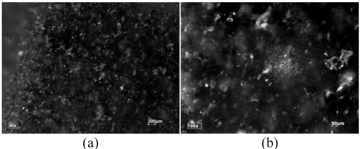
Figure 6. Stereomicrographs of PExp disperse in HTPB matrix. Magnification: A) 40x and B) 100x.
