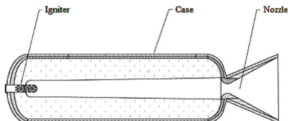
Figure 1. Components of a rocket motor<sup>15</sup>.
