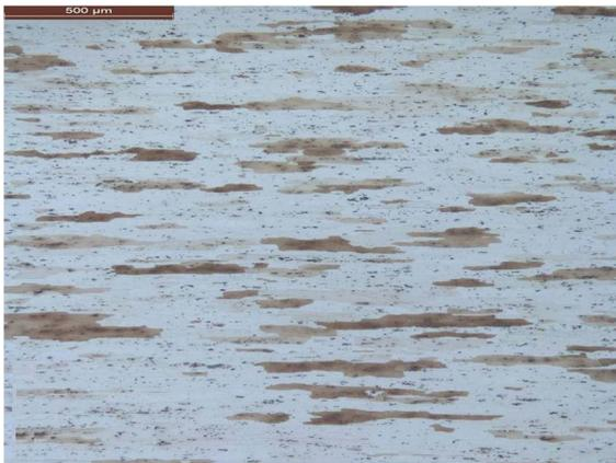
Figure 9. Aluminium alloy AA2024 as received.
