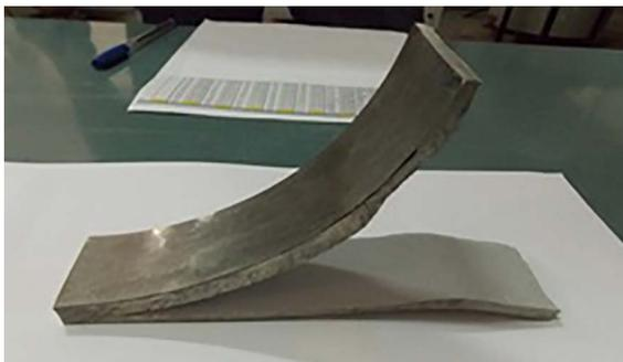
**Figure 3.** Commercial AA2024 aluminium alloy after 10 steps of cold rolling.
