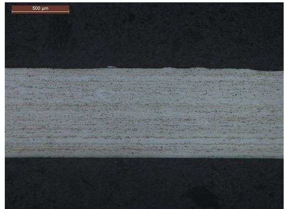
Figure 10. Aluminium alloy AA2024 cold rolled 90% 2h.
