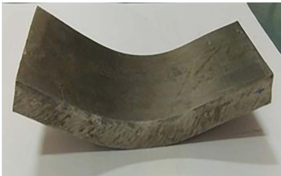
**Figure 2.** Commercial AA2024 aluminium alloy after 7 steps of cold rolling.
