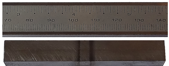
Figure 3. Simulated specimen (figure bottom part). The IC CGHAZ area is situated in the central part of the specimen and has the length of approximately 8 mm. Reference rule (figure top part) in mm
