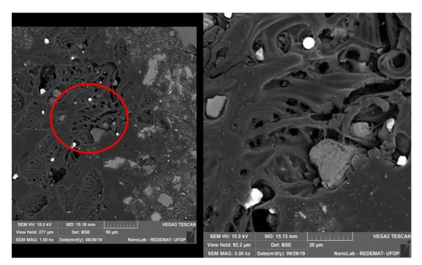
Figure 6. Micrograph of sample AF100-02 tested at 7 days with magnification of 1000x and 3000x.
