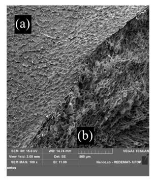
Figure 1. Fiber micrograph showing (a) frontal view of the epidermis of the fiber and (b) parenchymal region containing sclereids and parenchymal cells with lignified thickening bars.
