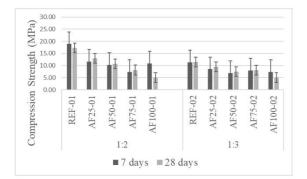
Figure 5. Compression Strength test results for 7 and 28 days.
