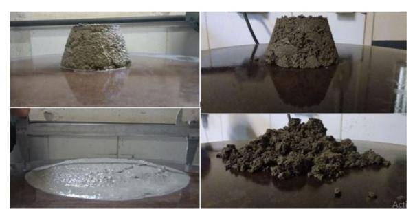
Figure 3. Comparison between the consistency of REF-02 and AF100-02 mortars.
