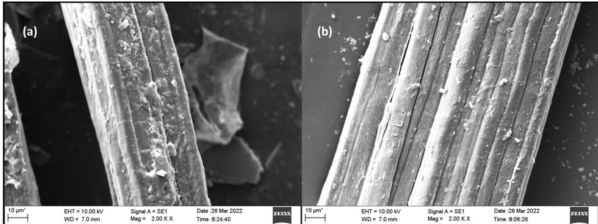
**Figure 2.** SEM Image of (a) untreated PALF (b) alkali treated PALF.
