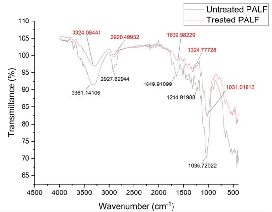
Figure 1. FTIR spectra of treated and untreated PALF fiber.
