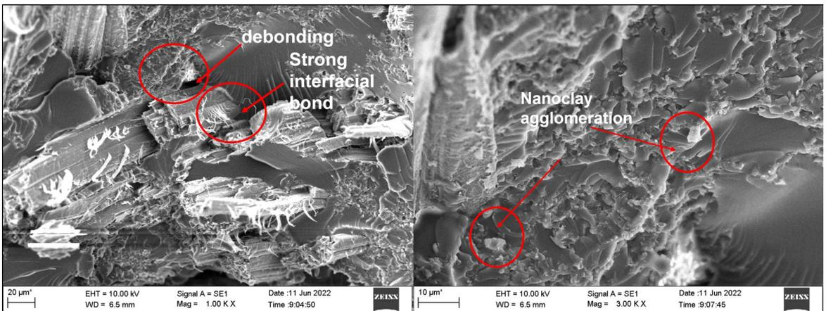
Figure 14. SEM images of P30NC3, (a) showing debonding in one area and strong interfacial bond in another area, (b) Matrix area showing nanoclay agglomeration.
