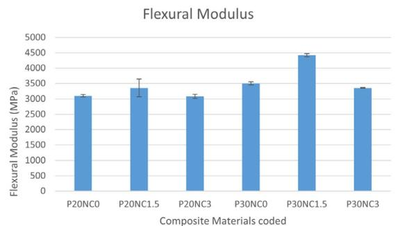
**Figure 9.** Flexural modulus of alkali treated PALF nanoclay epoxy composites.
