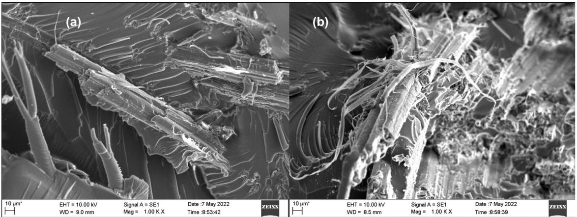
Figure 13. SEM images of P30NC1.5, (a) showing strong interfacial bonding, (b) showing fiber breakage or fracture.
