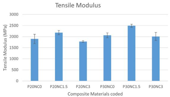
**Figure 7.** Tensile modulus of alkali treated PALF nanoclay epoxy composites.
