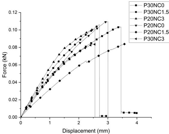
**Figure 5.** Force - displacement curves from flexural test for epoxy PALF composites with and without nanoclay.
