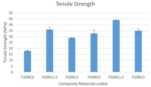
**Figure 6.** Tensile strength of alkali treated PALF nanoclay epoxy composites (P stands for PALF weight and NC stands for nanoclay weight percentage).
