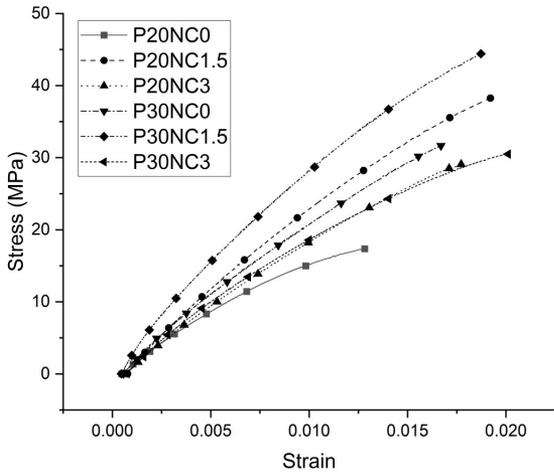
**Figure 4.** Stress-strain curve from tensile tests for epoxy PALF composites with and without nanoclay.
