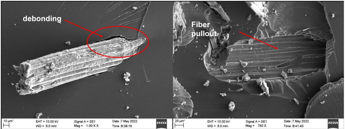
Figure 12. (a) SEM image of P30NC0 showing debonding at fiber matrix interface and (b) showing fiber pull-out.
