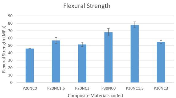
**Figure 8.** Flexural strength of alkali treated PALF nanoclay epoxy composites.
