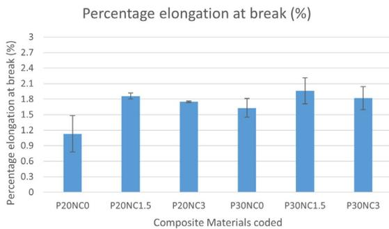
**Figure 10.** Percentage elongation at break (%) for different configurations of composite material.
