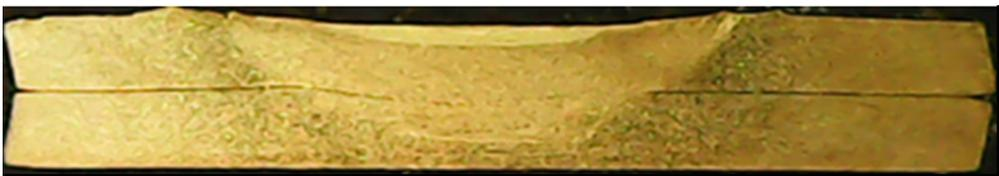
Figure 8. Cross section of lap joint processed with  $\omega = 1050$  rpm and  $v = 20$  mm/min.
