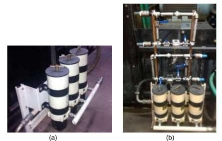
Figure 2. PIUSI fuel meter placement – entrance side: (a) before installation, and (b) after the installation.
