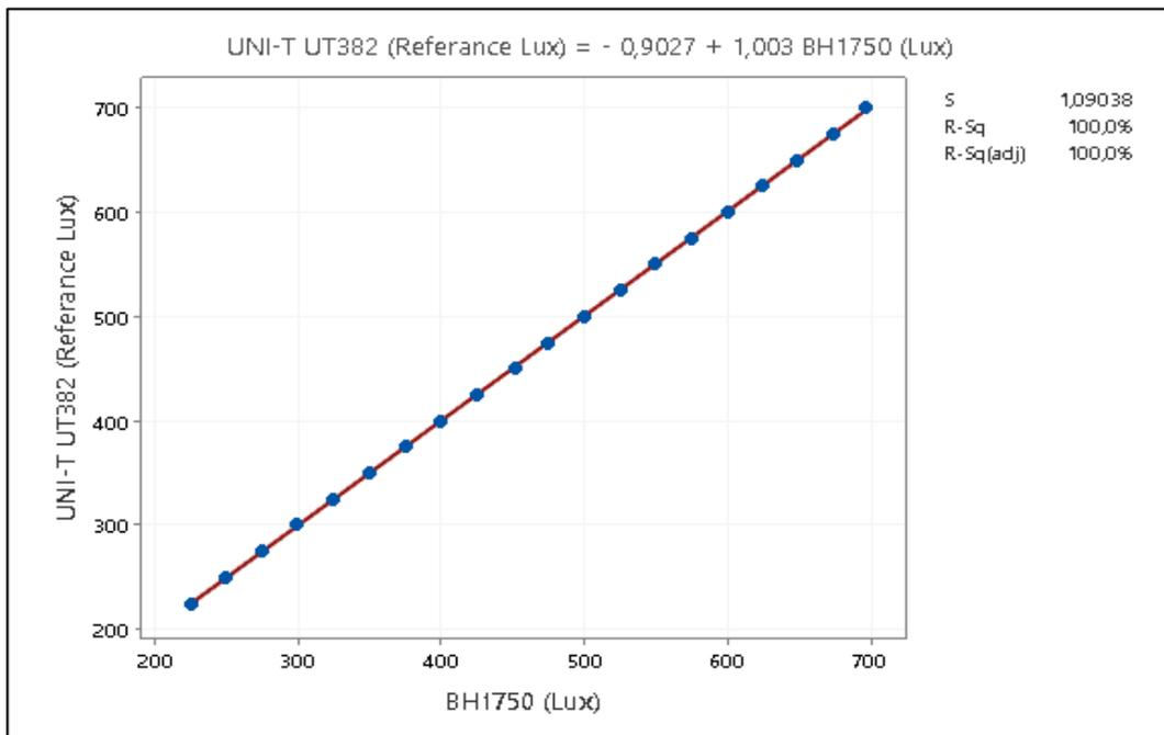
**Figure 13.** Regression equation and coefficient based on UNI-T UT382 vs. BH1750 for the measurement
