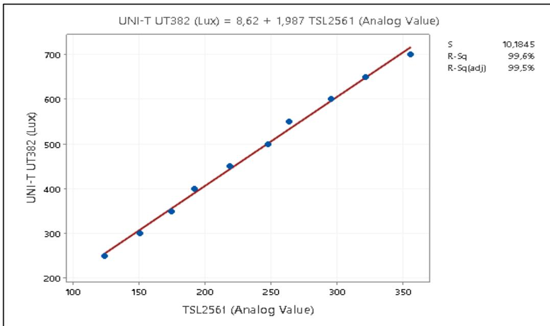
**Figure 9.** Regression equation and coefficient based on UNI-T UT382 vs. TSL2561 for the calibration
