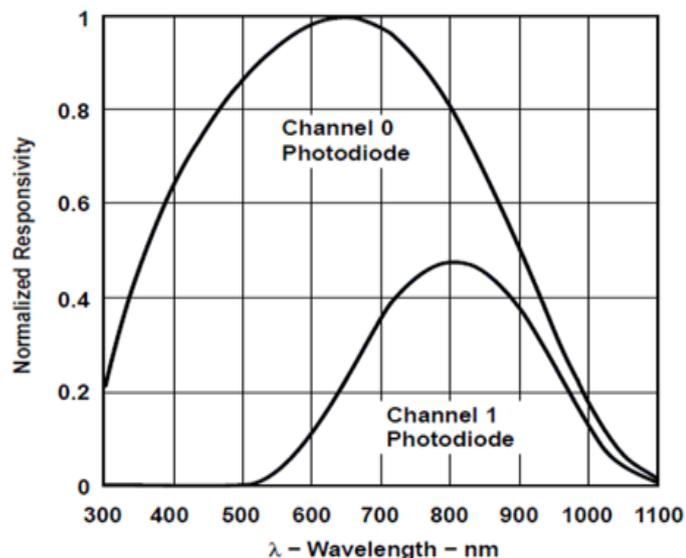
Figure 2. The spectral responsivity of the TSL2561 sensor [19]
