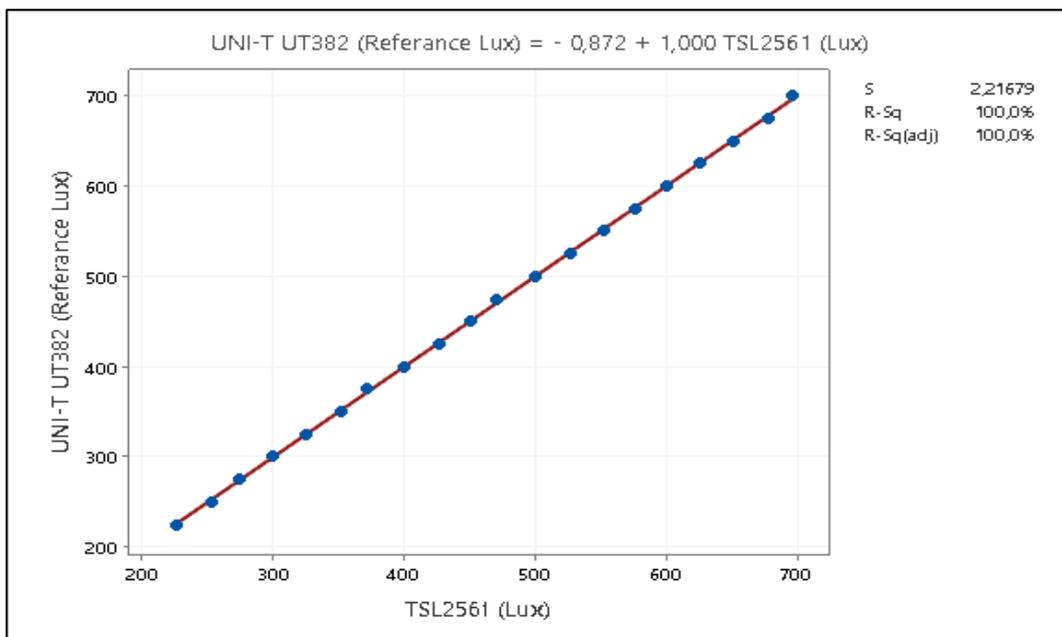
**Figure 12.** Regression equation and coefficient based on UNI-T UT382 vs. TSL2561 for the measurement
