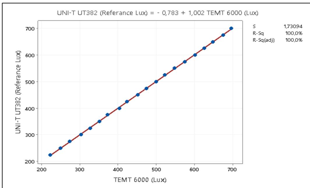
**Figure 14.** Regression equation and coefficient based on UNI-T UT382 vs. TEMT6000 the measurement.
