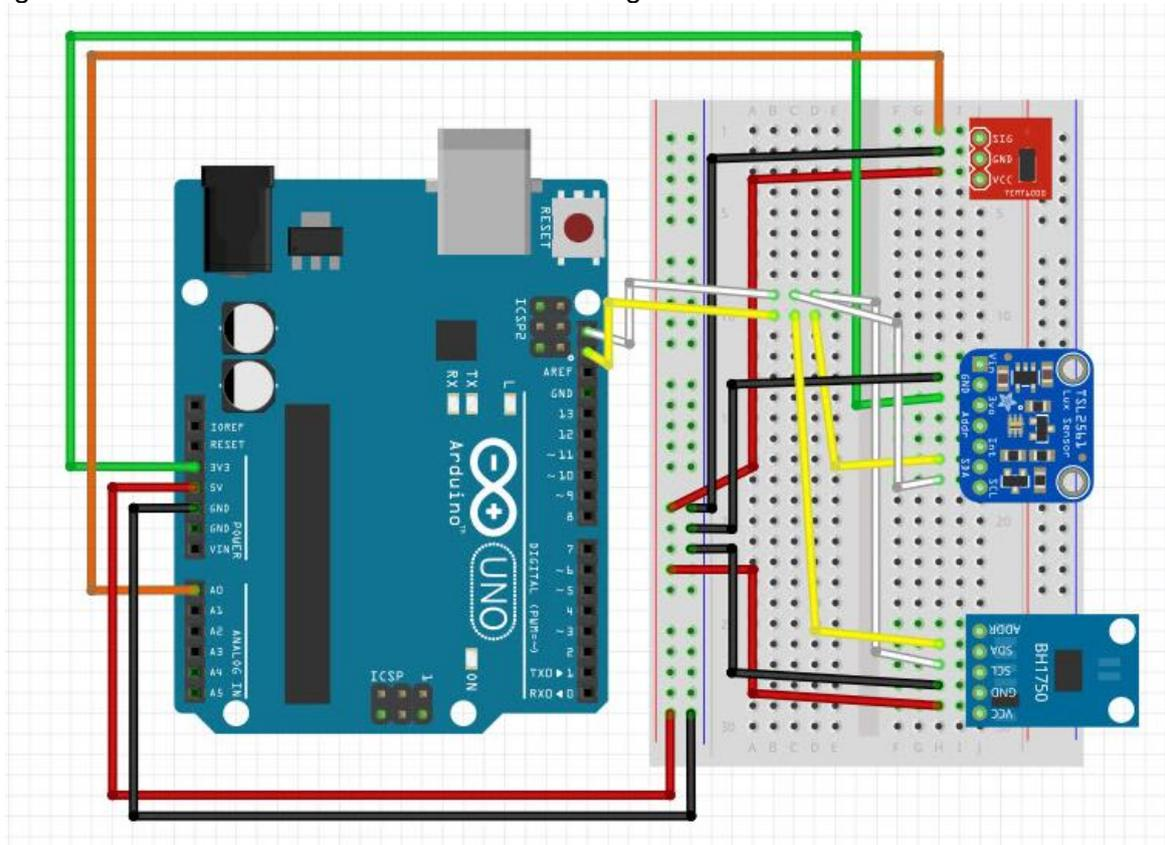
**Figure 7.** Wiring diagram of low-cost sensor connections with Arduino UNO
