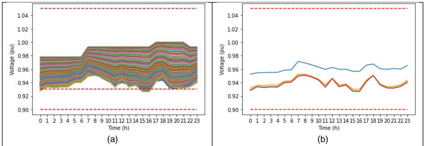
**Figure 2.** (a) Voltage for all buses; (b) Voltage for GLD buses.
