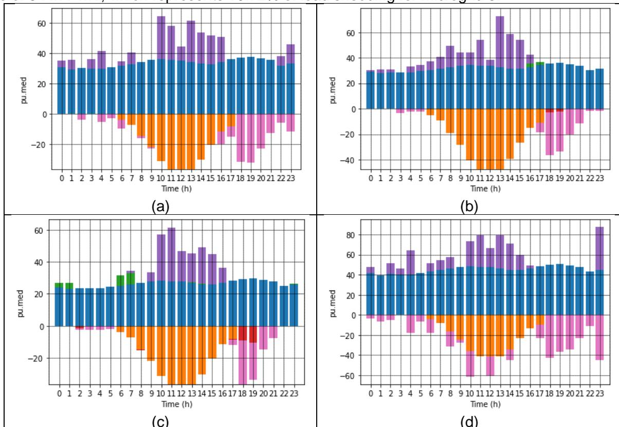
**Figure 3.** MOUG optimization dispatch in case II for microgrids (a) 1, (b) 2, (c) 3, and (d) 4. NC-load in blue; C-load in purple, battery charge in green; battery discharge in red; PV-gen in red.
