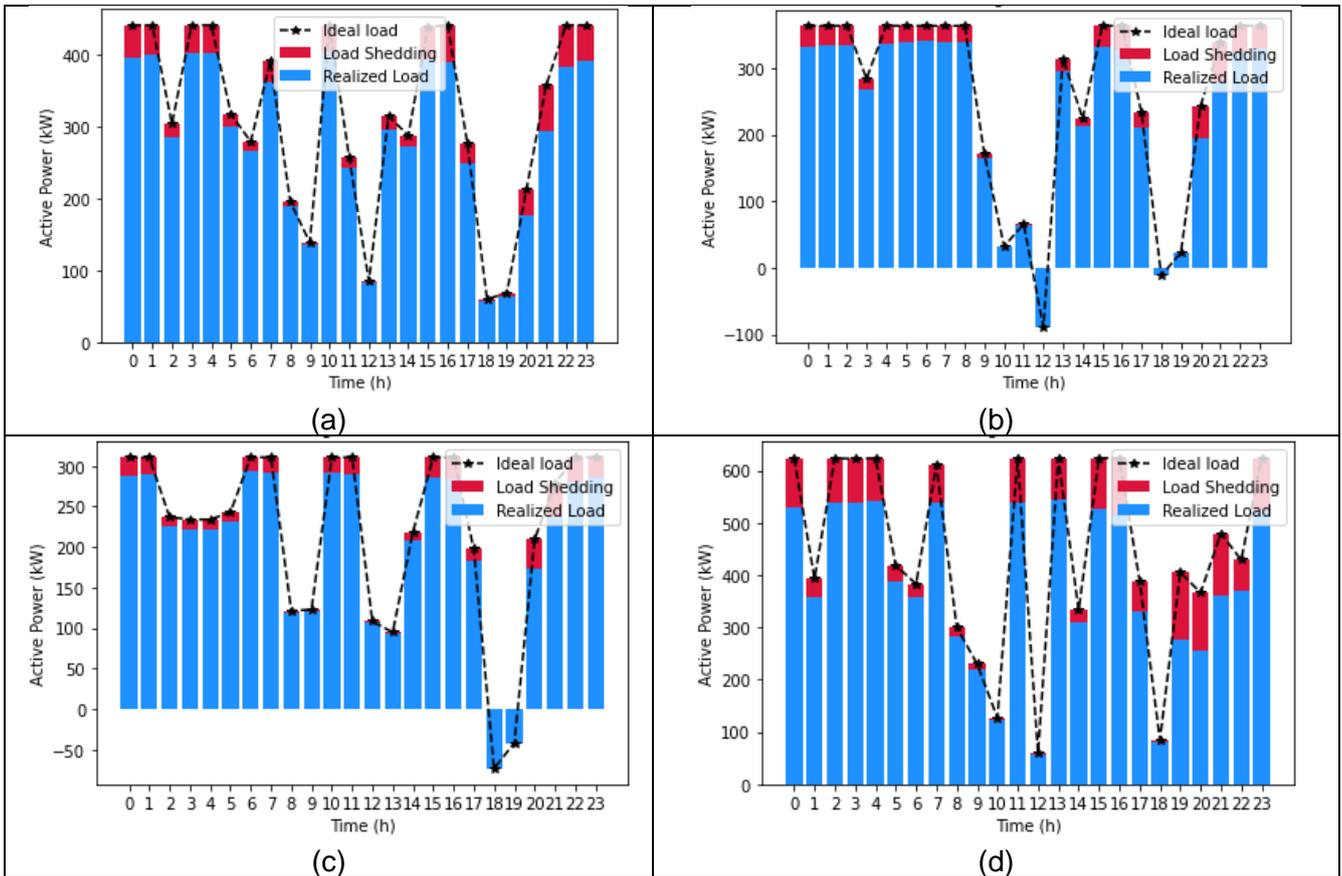
Figure 7. Ideal power injection from the main grid point of view for microgrids (a) 1; (b) 2; (c) 3; and (d) 4.
