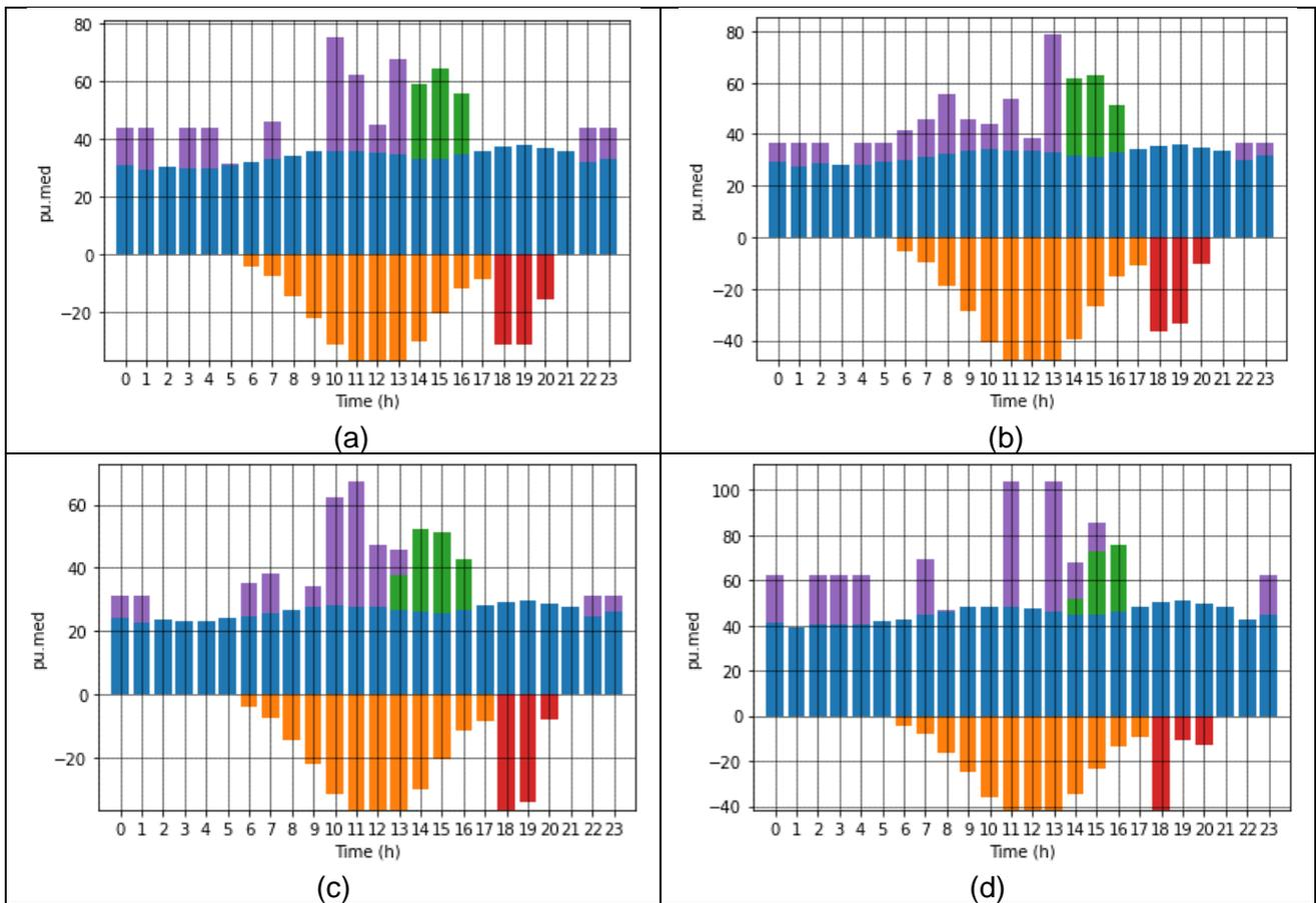
**Figure 1.** MOuG optimization dispatch during pre-processing for microgrids (a) 1, (b) 2, (c) 3, and (d) 4. NC-load in blue; C-load in purple, battery charge in green; battery discharge in red; PV-gen in orange.
