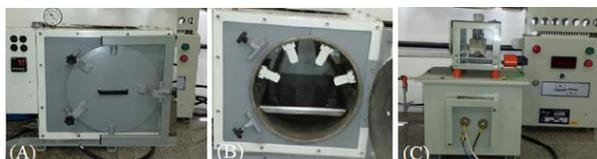
**Figure 2:** (a,b) UV chamber; (c) Corona Treatment Station.
