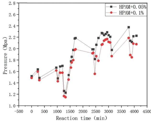
Figure 8: The changes of outlet pressures in complex drive experiment of oil sand.
