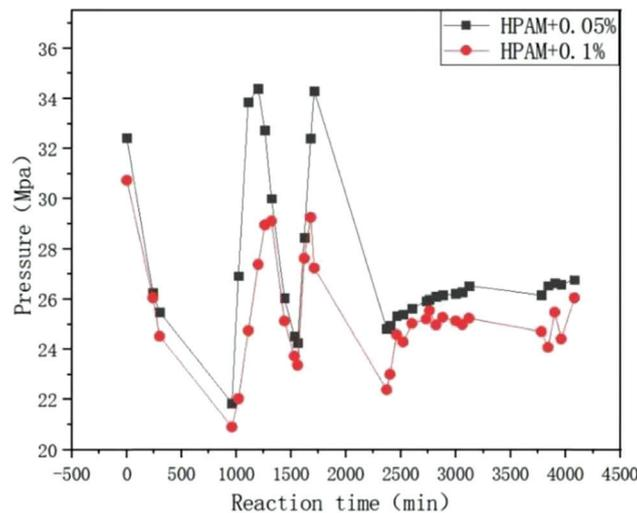
Figure 9: The changes of pressure difference in complex drive experiment of oil sand.
