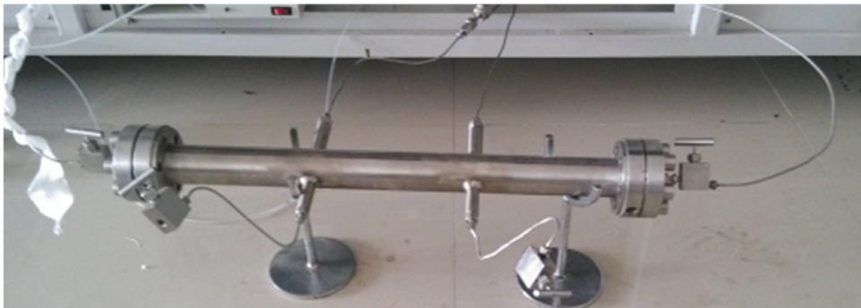
**Figure 6:** Sand filling pipe.
