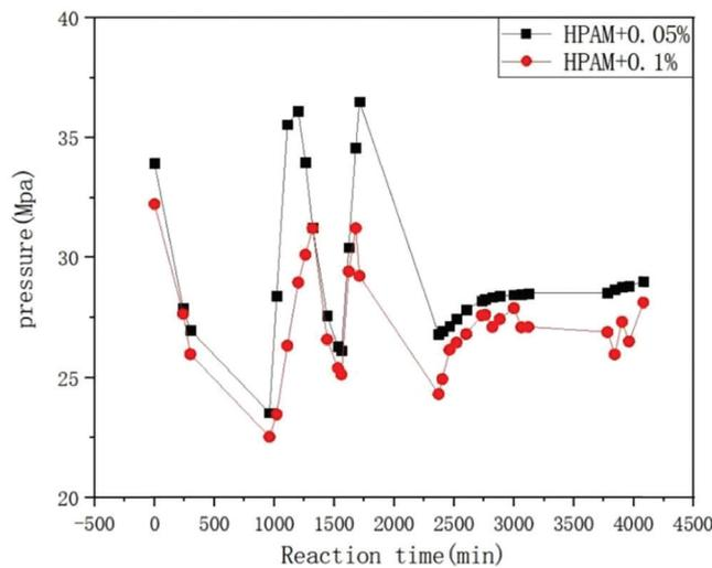
**Figure 7:** The changes of entrance pressures in complex drive experiment of oil sand.
