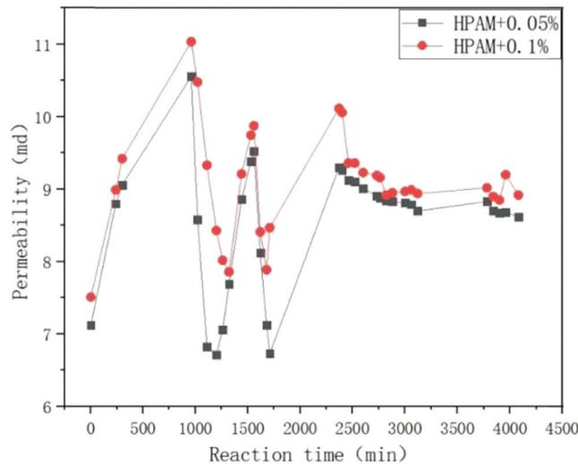
**Figure 10:** The changes of Permeability in complex drive experiment of oil sand.
