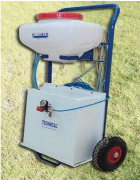
Figure 2. The injection device recommended by MEWA, Saudi Arabia to control R. ferrugineus .
