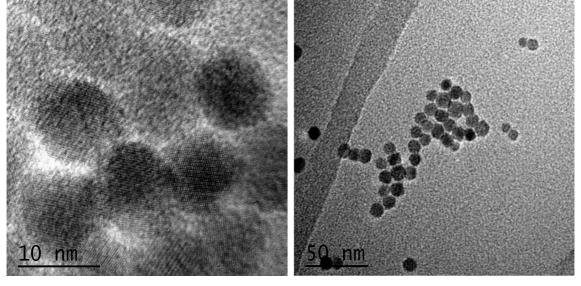
Figure 1. View of Selenium Nanospheres by Transmission Electron Microscopic (a) 10nm scale bar (b) 50nm scale bar with magnified form.
