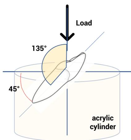
**Figure 1.** Load was applied at an angle of  $135^\circ$  to the long axis of the root.
