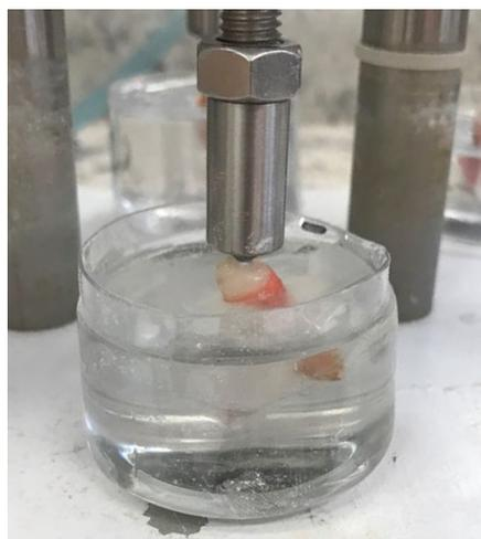
**Figure 2.** Specimen being cycled in the Biocycle-Piopdi cyler (São Carlos, SP, Brazil).
