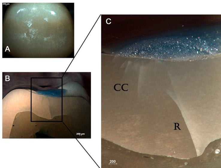
**Figure 6-** A) Occlusal damage in LD crown (0.8x). B) Side view of LD crown (0.8x). C) Side view (2.5x) showing partial cone (CC) and flexure-induced radial (R) cracks
