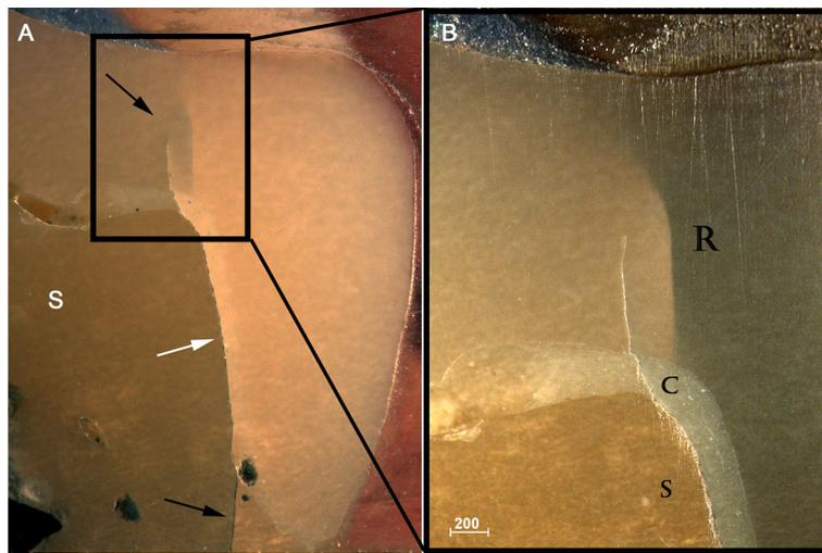
**Figure 8-** A) Side view (1,6x) of RNC crown showing a radial crack that propagated up- and downwards (black arrows) through the interface (white arrow) of composite substrate (S) and resin cement. B) 2.5x magnification showing the radial crack (R), cement (C) and composite substrate (S)
