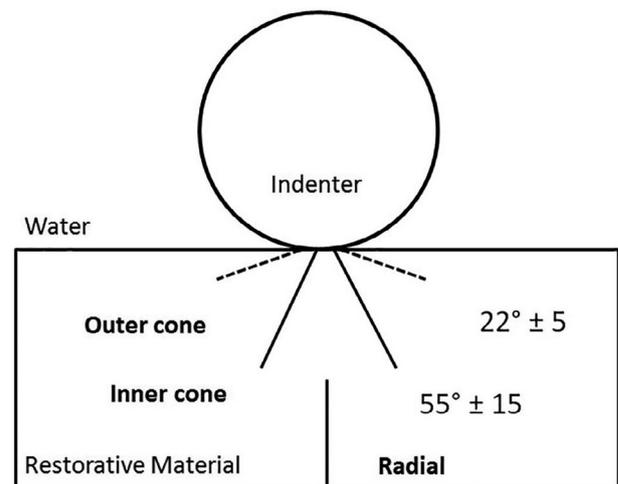
**Figure 3-** Schematic of contact damage. Outer cone cracks originate around the contact area and typically present an angle of  $22 \pm 5^\circ$  relative to free surface. For inner cone cracks, the measure is  $55 \pm 15^\circ$ . Radial cracks originate from the cementation surface and propagate sideways and upwards. Viewed from below, they are star-shaped. However, from side view we can identify one of its arms propagating towards the contact area
