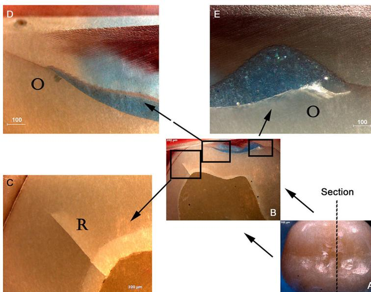
**Figure 9-** Damage modes in RNC crowns. A) Occlusal view (0,8x) whose section is shown in B. B) Side view that is shown in high magnification. In C (4x) we identify a flexure induced radial crack (R) on buccal face. D and E (4x) show outer cone cracks around indentation area
