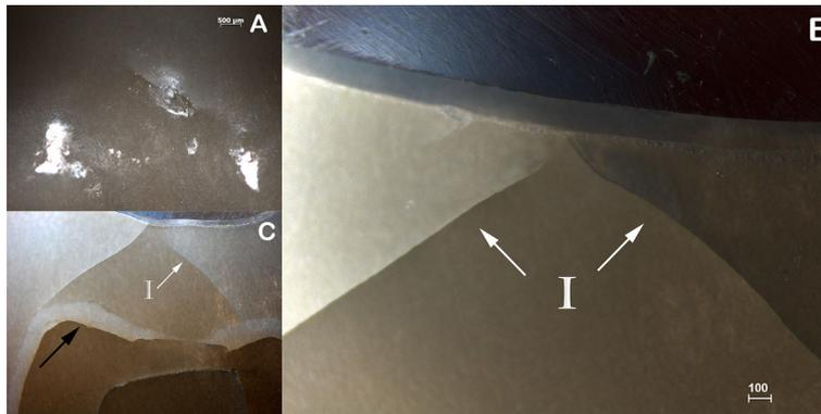
**Figure 5-** A) Occlusal damage in LD crown (1.25x). B) On the side view of the polished specimen (4x), subsurface damage analysis showed contact-induced inner cone cracks (I). C) Inner cone cracks extending to the cementation surface (I), black arrow shows resin cement layer (1.6x)
