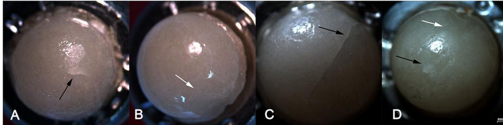
**Figure 11-** Lithium disilicate indenters (0,8x) A and B loaded LD crowns, C and D loaded RNC crowns. A) Black arrow show small contact crack. B) White arrow show chipping starting in the fixture base. C) Black arrow shows large crack that started in fixture base. D) Black arrow shows removal of glaze, white arrow show chipping starting in the fixture base
