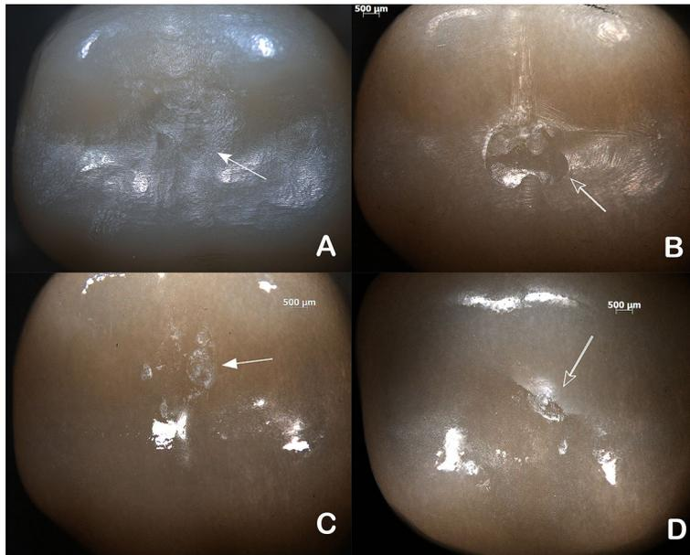
**Figure 4-** Occlusal view of surface damage after 2 million cycles (0.8x). Small (A) and large (C) wear facets in RNC crowns cycle. Wear facets (C) and crack (D) in LD crowns after 2 million cycles
