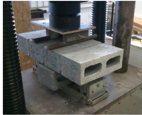
(b) Loading through hydraulic press
