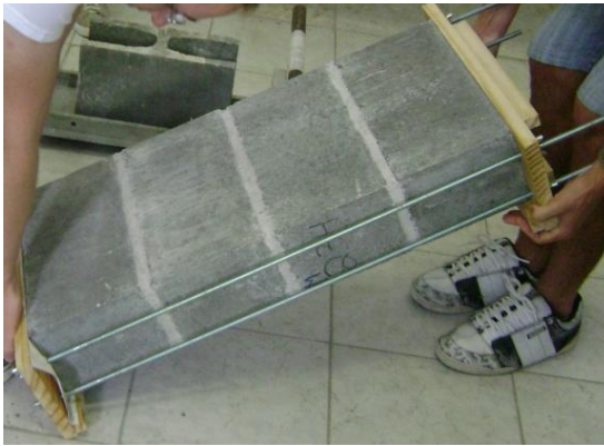
(a) Confining support for handling the prisms
