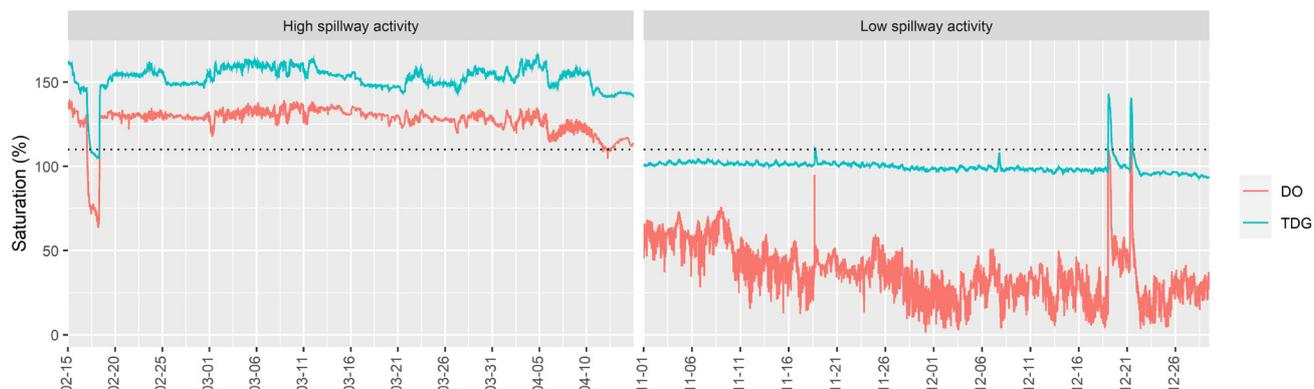
**FIGURE 3** | Saturations of dissolved oxygen (DO, red) and total dissolved gases (TDG, blue), for periods with intense (left) and sporadic (right) dam spillway activities. The black dotted line indicates the threshold of 110% TDG saturation.
