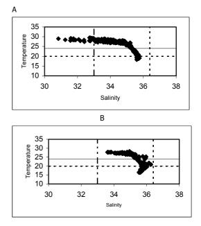
Fig. 2. Scattered T-S diagrams for the São Sebastião area, from west site (A) and southeast and south (B), during summer 1994. Vertical and horizontal lines delimit the water masses described in the text: Temperature > 24 and Salinity < 33= Coastal Water; Temperature > 20 and Salinity > 36.4= Tropical Water; Temperature < 20 and Salinity > 36.4 = South Atlantic Central Water.
