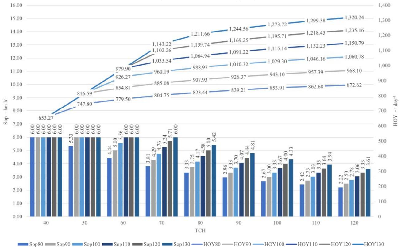
**Figure 5** - Comparison of cost related to mechanized cutting of sugarcane in 1.50 m spacing, 0.90 m x 1.40 m spacing, dual-row simultaneous harvest in 1.50 m spacing
