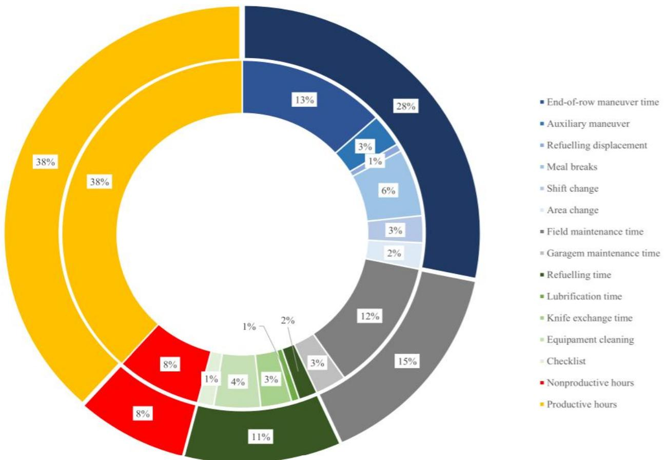
Figure 11 - Pareto diagram for offenders of mechanized harvest
