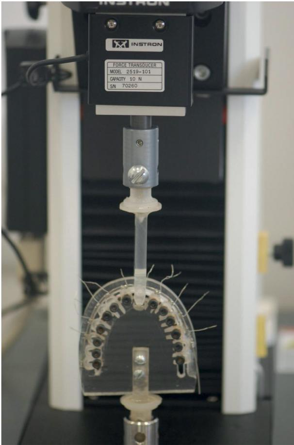
**Figure 2.** Tip of the Universal testing machine applying a bucco-lingual pressure to the acrylic structure.
