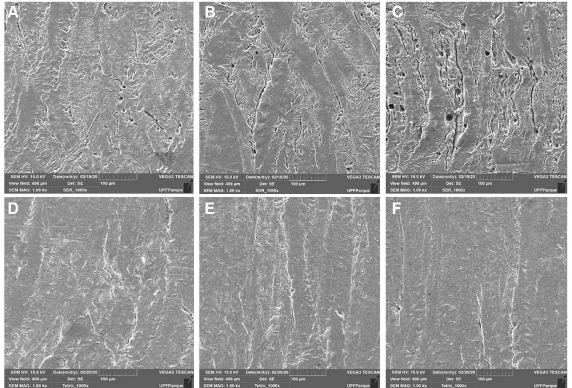
**Figure 3.** Scanning electron microscopies (1000x) of Bulk fill Flow SDR (A, B, C) and Tetric N-Ceram Bulk fill (D, E, F) composite resins in the superficial (A, D), middle (B, E) and cervical (C, F) thirds of the proximal wall after acid challenge.
