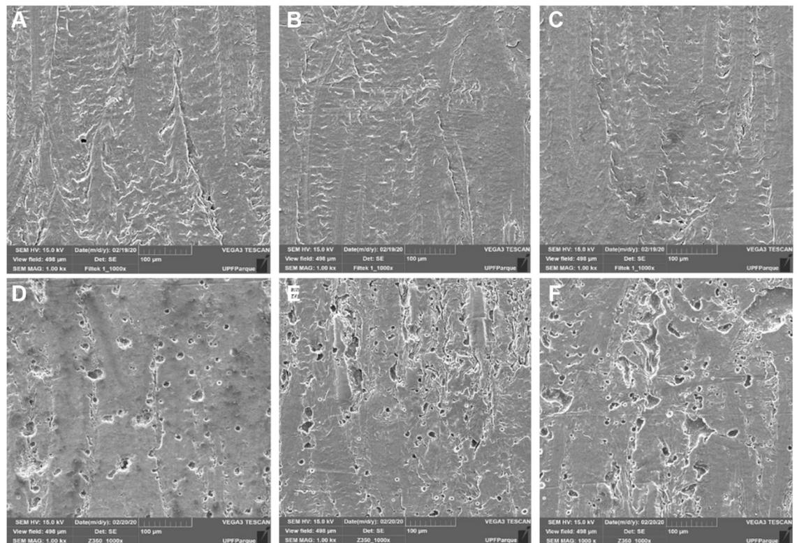
**Figure 4.** Scanning electron microscopies (1000x) of Filtek Bulk fill (A, B, C) and Filtek Z350 XT (D, E, F) composite resins in the superficial (A, D), middle (B, E) and cervical (C, F) thirds of the proximal wall after acid challenge.
