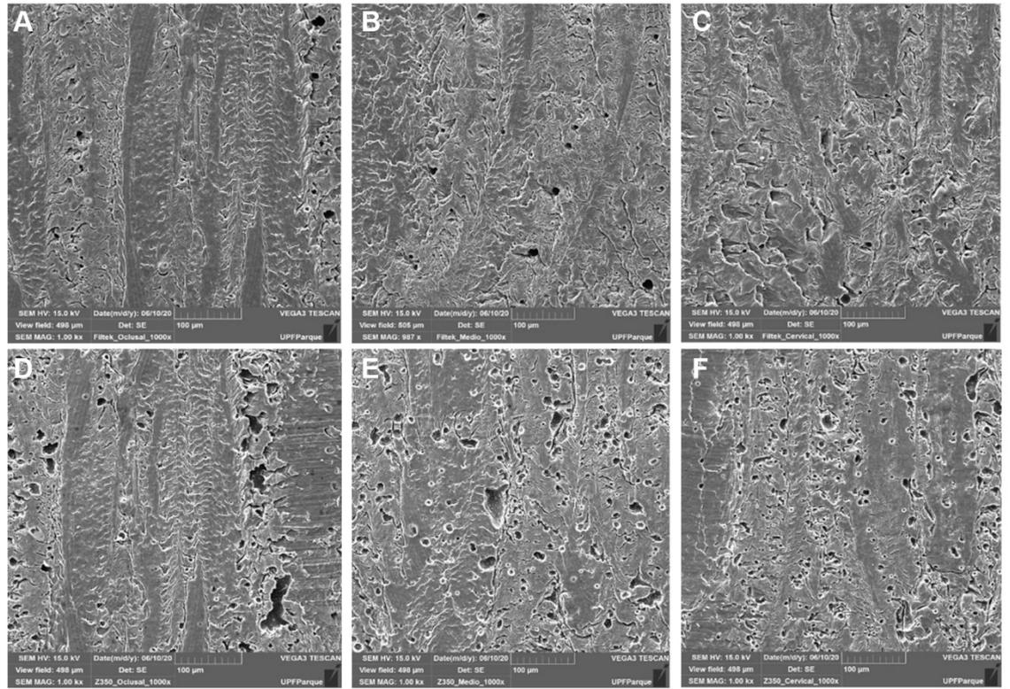
**Figure 2.** Scanning electron microscopies (1000x) of Filtek Bulk fill (A, B, C) and Filtek Z350 XT (D, E, F) composite resins in the superficial (A, D), middle (B, E) and cervical (C, F) thirds of the proximal wall before acid challenge.
