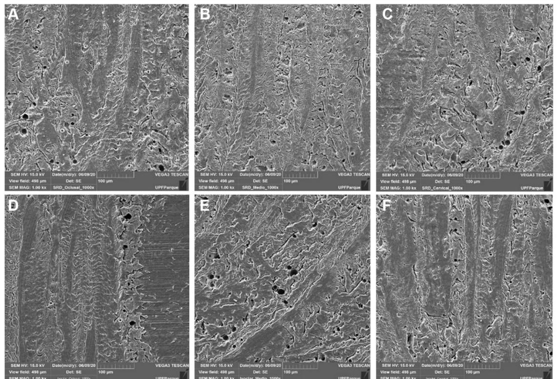
**Figure 1.** Scanning electron microscopies (1000x) of Bulk fill Flow SDR (A, B, C) and Tetric N-Ceram Bulk fill (D, E, F) composite resins in the superficial (A, D), middle (B, E) and cervical (C, F) thirds of the proximal wall before acid challenge.
