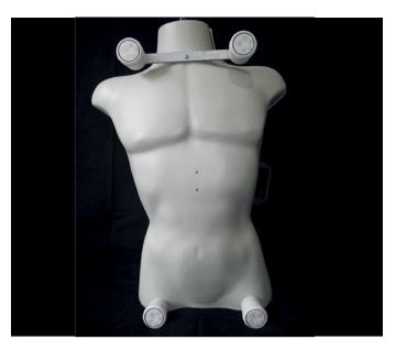
Figure 2. View of the anterior portion of the mannequin, with the four levelling feet attached.
