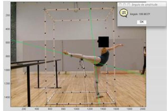
**Figure 2.** Example in how angle between body segments were obtained; asterisks represent the anatomical points marked for obtain the angle between body segments in this technical skill (*arabesque*). For each technical skill were marked different anatomical points.
