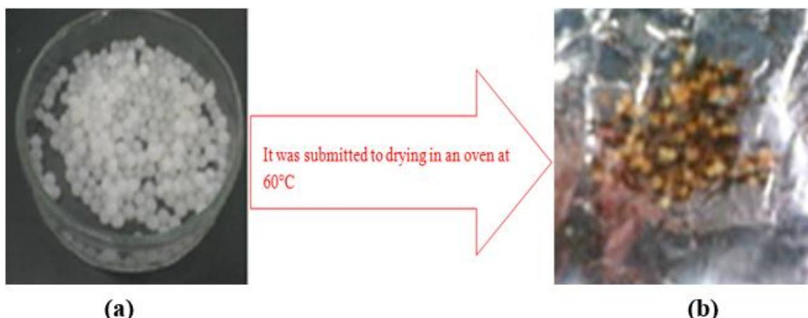
**Figure 3.** Illustration of the encapsulation of alginate / Capsul® and nutrients (N and P) obtained before (a) and after drying in an oven at 60°C (b).
