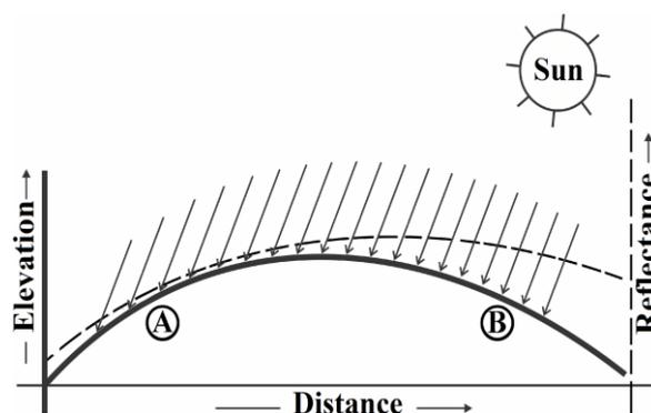
**Figure 1:** A schematic diagram illustrating the variation of reflectance on Landsat spectral data as function of topography and illumination effects. A: Slope facing away from the sun (weakly illuminated area); B: Slope facing to the sun (well-illuminated area). Source: Modified from Moreira (2014).
