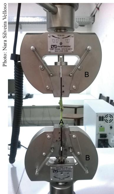
Figure 3. Crimping of a rachilla sample (A) between the two grips (B) of the Instron 3365 universal testing machine used for the traction test, with 5 cm between grips.
