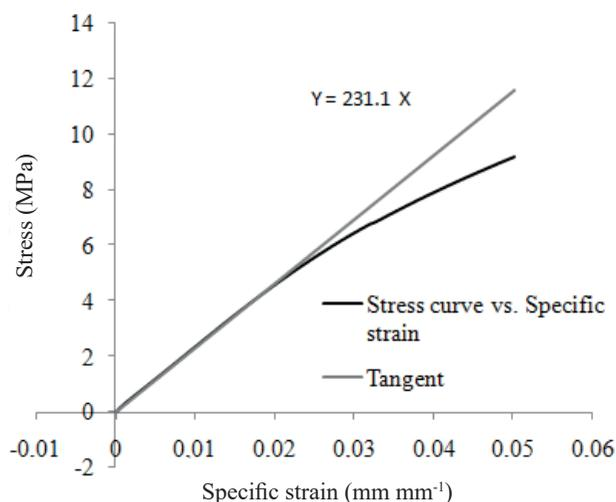
Figure 5. Stress curve and specific strain and its tangent, obtained experimentally for macaw palm rachilla in the mature stage.
