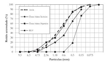
Figure 2 Fine aggregate and RLV particle size curve
