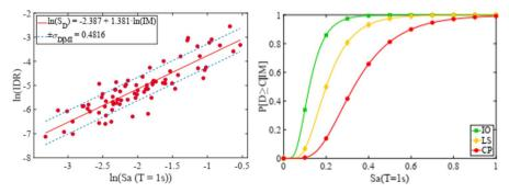
Figure 6. Probabilistic Seismic Demand Model (PSDM) (left) and fragility functions (right) of the analyzed RC structure.
