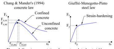
Figure 4. Generic representation of concrete and steel material law.
