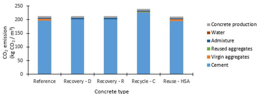
**Figure 3.** CO<sub>2</sub> emission levels for compressive strength class C30 concretes.
