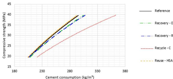
**Figure 2.** Concrete mixing design curves.
