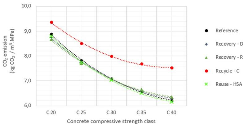
Figure 5. CO<sub>2</sub> emission per MPa of 1 m<sup>3</sup> of concrete with 100 mm slump, vs. concrete compressive strength.
