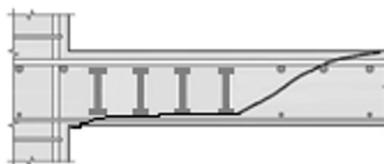
Figure 3: Crack delamination patterns.
