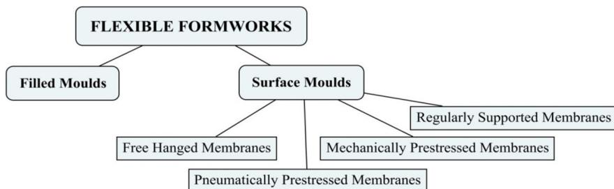
**Figure 23.** Proposal for flexible formworks categorization into families [46].
