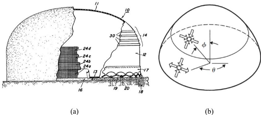
**Figure 10.** (a) Improvements to Neff system - Adapted from [25] and (b) identification of the horizontal rupture plane, which in the case of spherical shell corresponds to  $\phi = 51,5^0$  - Adapted from [4].
