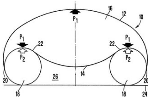
**Figure 14.** Design of a secondary pneumatic enclosure at the base of the membrane. Adapted from [28].
