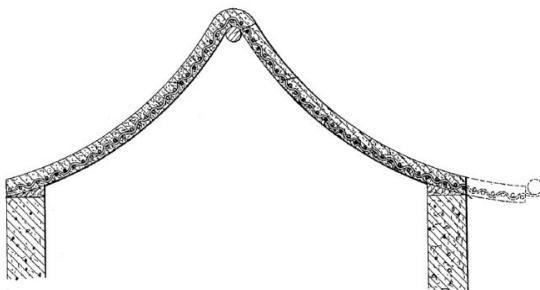
**Figure 4.** A coverage produced with a fabric mould. Adapted from [10].
