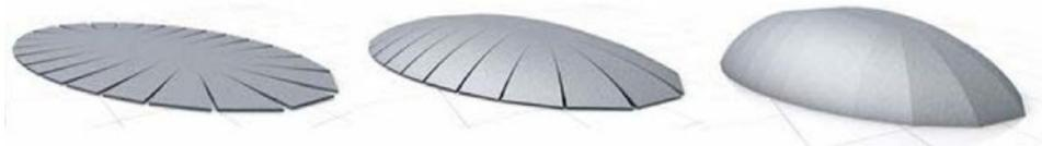
**Figure 25.** “Pneumatic Forming of Hardened Concrete (PFHC)” construction process. Adapted from [30].
