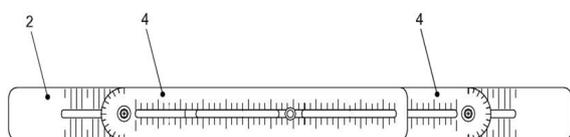
**Figure 4.** Enlarged lateral detail of the inter-ruler joint of the abdominoplasty marking instrument. Perspective view of the abdominoplasty marking instrument in transport position.
