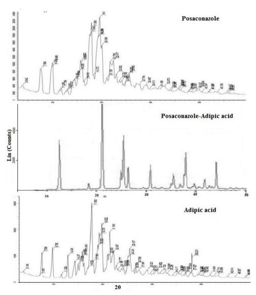
FIGURE 2 - PXRD pattern of posaconazole-adipic acid co-crystal and its individual components.
