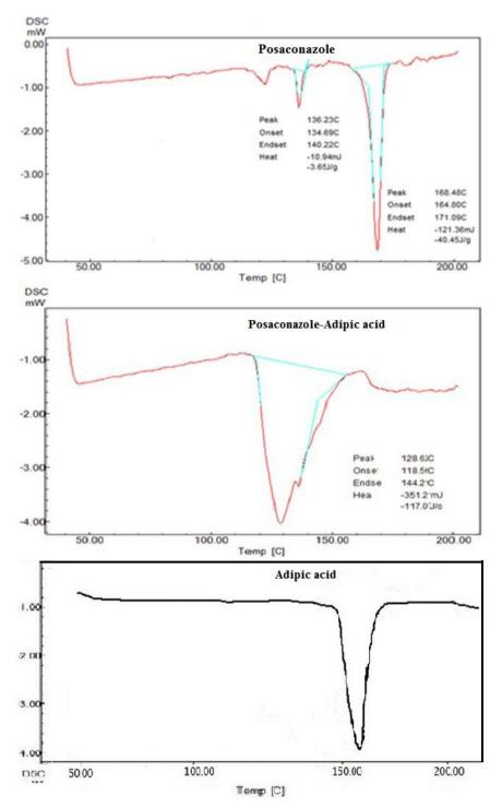
FIGURE 3 - DSC thermogram of posaconazole, posaconazole-adipic acid co-crystals and adipic acid.
