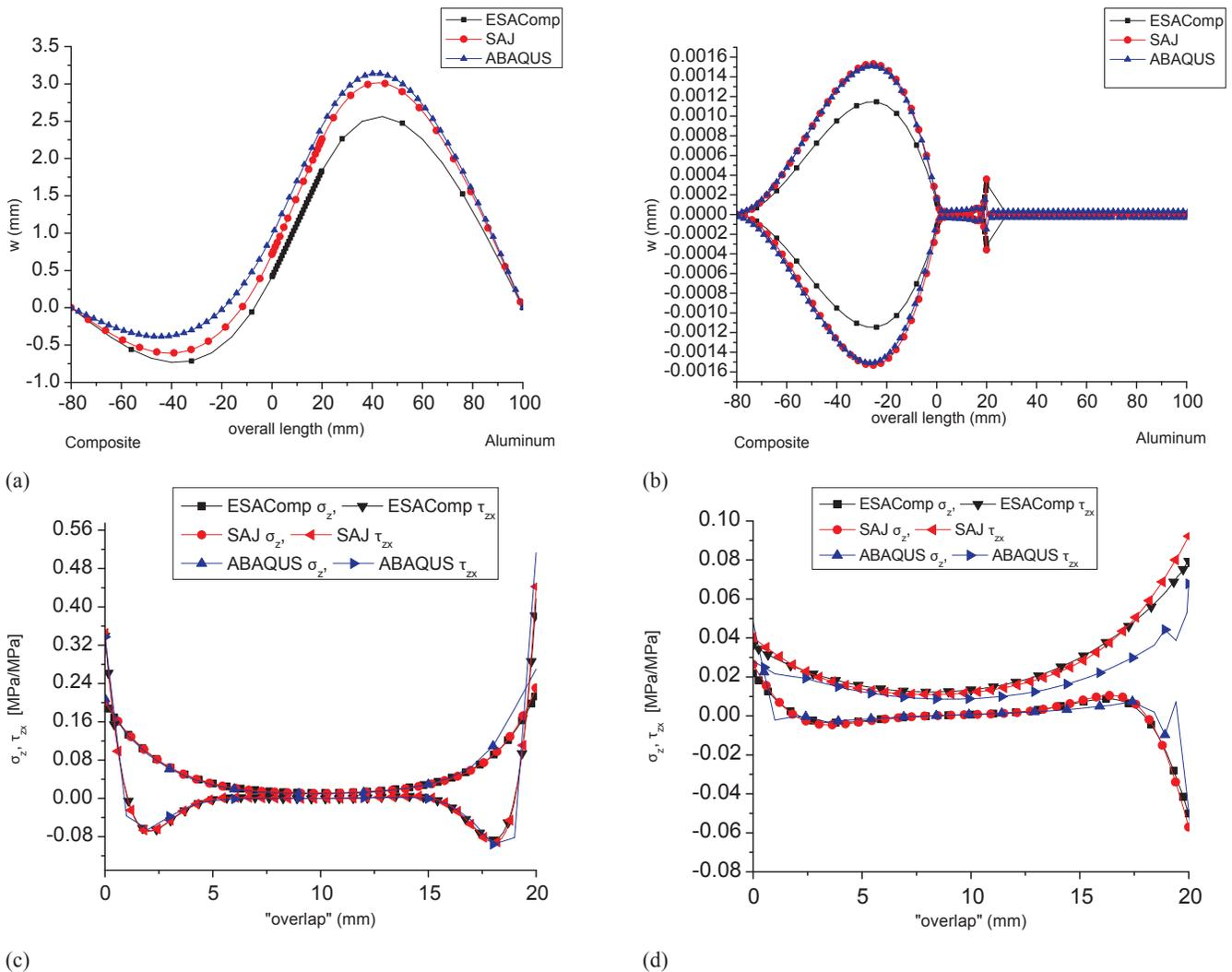
Figure 7. (a) Single lap hybrid joint displacement in  $w$  direction; (b) double lap hybrid joint displacement in  $w$  direction; (c) normalized single lap joint  $\sigma_{az}$  and  $\tau_{ax}$ ; (d) normalized double lap joint  $\sigma_{az}$  and  $\tau_{ax}$ .
