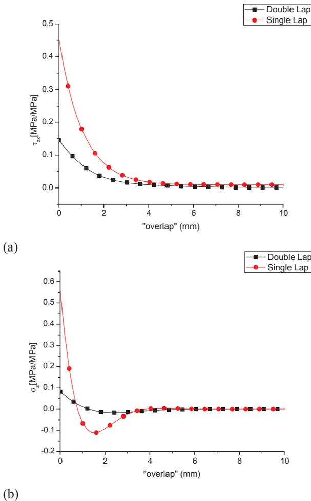
Figure 9. Single vs. double lap joint (half of the overlap length): (a) normalized  $\tau_{xz}$  shear stress in plane  $zx$ ; (b) normalized  $\sigma_z$  normal stress in  $z$  direction.
