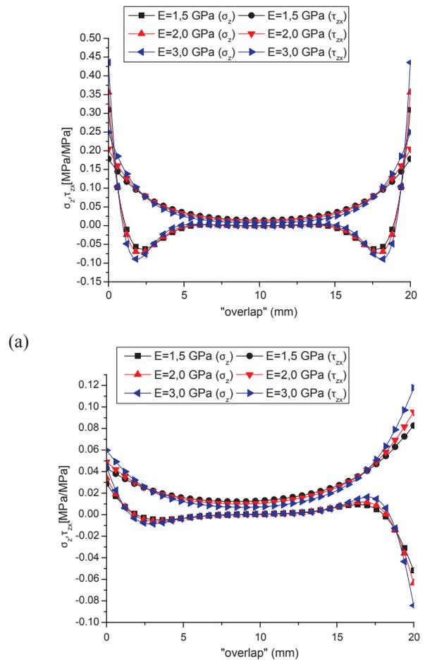
Figure 10. Young modulus: (a) single lap joint; (b) double lap joint.
