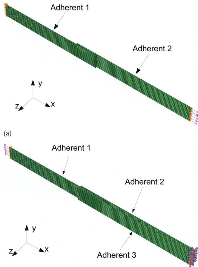
Figure 5. Finite element model: (a) single lap joint; (b) double lap joint.
