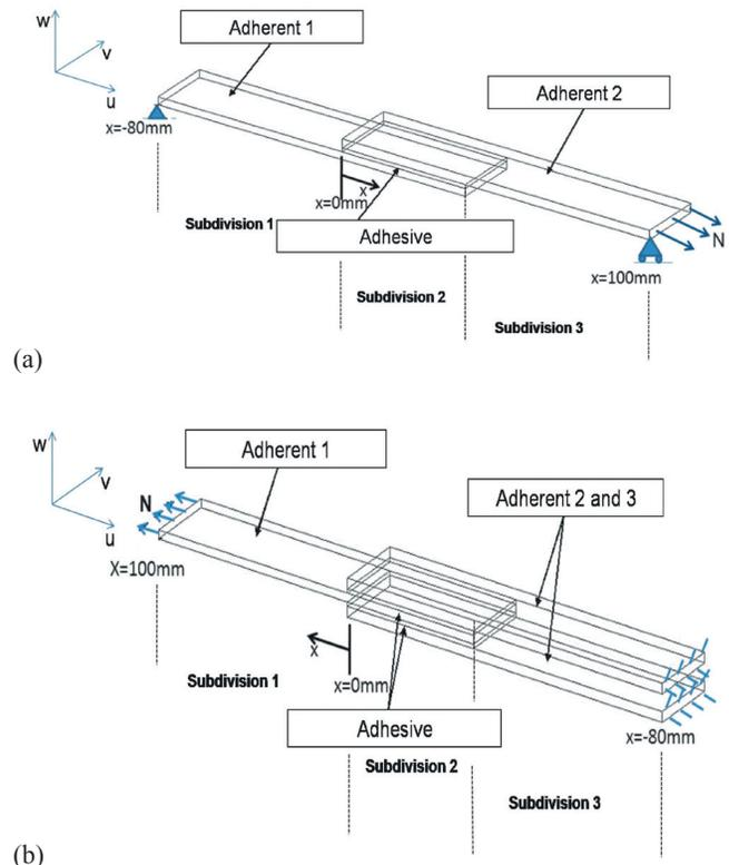
Figure 1. Boundary conditions, loads and coordinate system: (a) single lap joint; (a) double lap joint.
