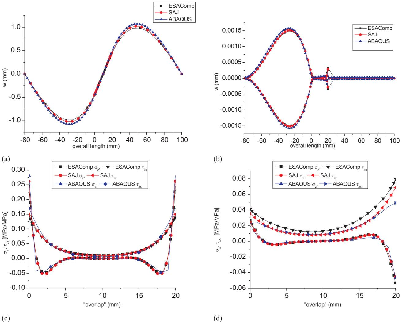
Figure 6. (a) Single lap composite joint displacement in  $w(z)$  direction; (b) double lap composite joint displacement in  $w(z)$  direction; (c) normalized single lap joint  $\sigma_{zz}$  and  $\tau_{zx}$ ; (d) normalized double lap joint  $\sigma_{zz}$  and  $\tau_{zx}$ .
