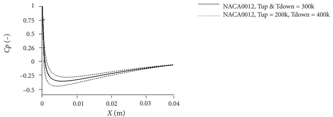
**Figure 11.** Pressure coefficient for NACA0012 airfoil at  $Re = 3000$ .
