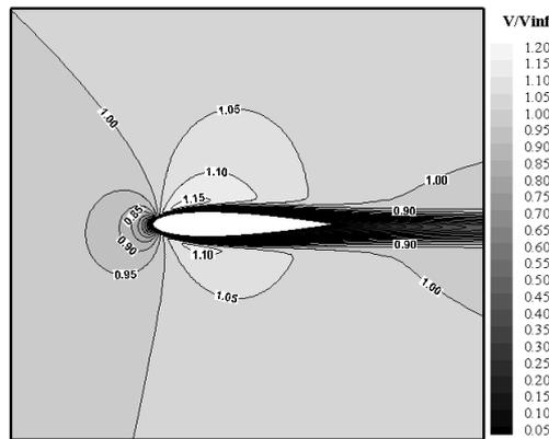
**Figure 9.** Velocity contour around NACA0012 airfoil at  $Re = 3000$  and  $T_u = 200$  K and  $T_l = 400$  K.
