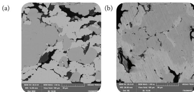
**Figure 9.** SEM microstructure (1500 $\times$ ) obtained for compounds III (a), and V (b).
