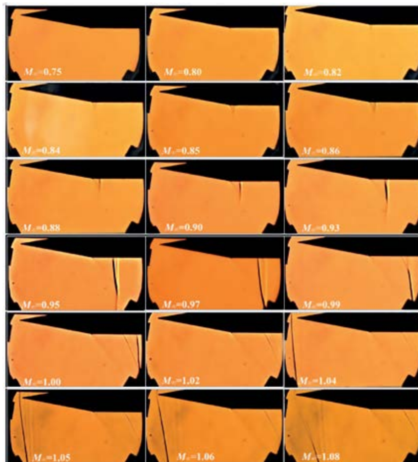
Figure 8. Schlieren images for model cone-cylinder forebody with blockage area ratio of 0.78%, for stagnation pressure of 80 kPa and stagnation temperature of about 300 K.
