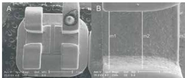
**Figure 1** - Scanning Electron Microscopy image of a bracket pertaining to Group III - (A) magnification at 50x and (B) 230x. The lines m1, m2 and m3 are the regions where the measurements were done to calculate slot height. The large variation of bracket dimensions can be observed, especially on mesial and distal ends.
