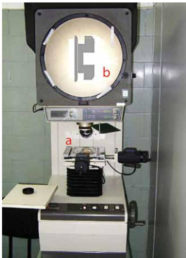
**Figure 2** - Profile projector. (a) Once the brackets were correctly positioned on this device, their shadows were projected with a substantial magnification. (b) Bracket height and depth were measured.
