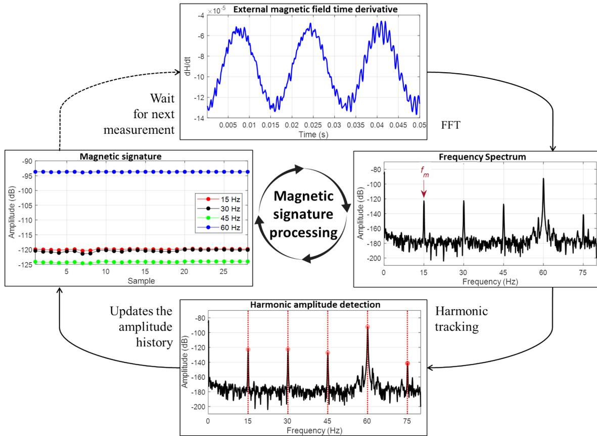
Fig. 4. Magnetic signature processing for a 8-pole synchronous generator operating at 60 Hz.
