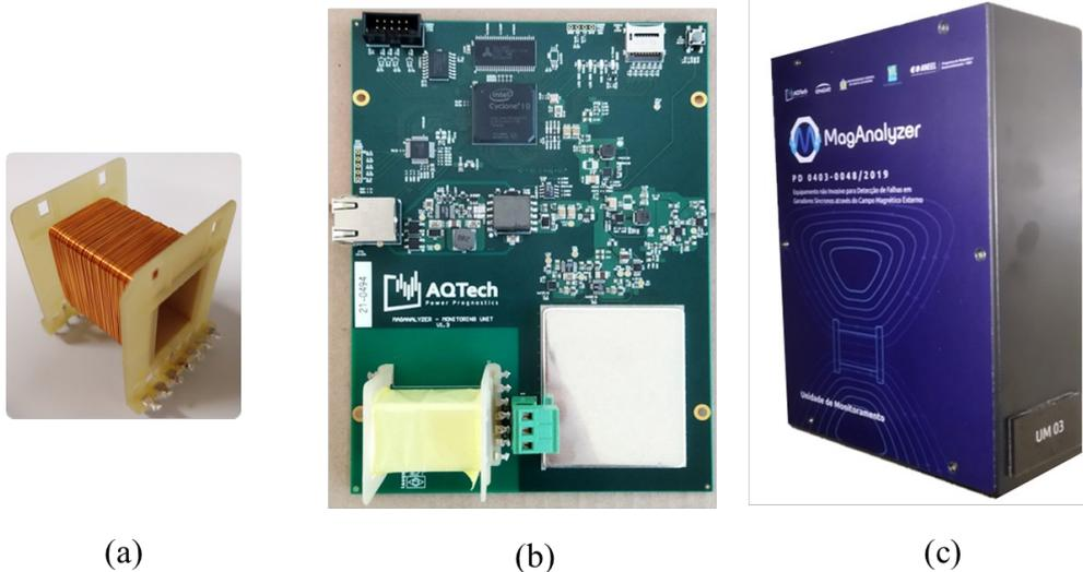
Fig. 10. Monitoring unit: (a) induction field sensor, (b) MU circuit board, (c) MU cabinet.
