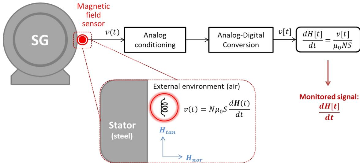
Fig. 2. General architecture for measuring the external magnetic field time derivative.
