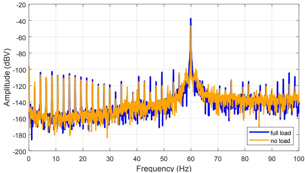
Fig. 17. Change of the frequency spectrum with increasing load on the SG.
