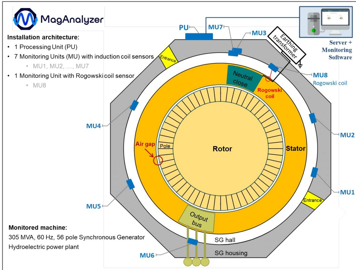
Fig. 14. Positioning of the MagAnalyzer elements installed in a 305 MVA SG of a hydroelectric power plant.
