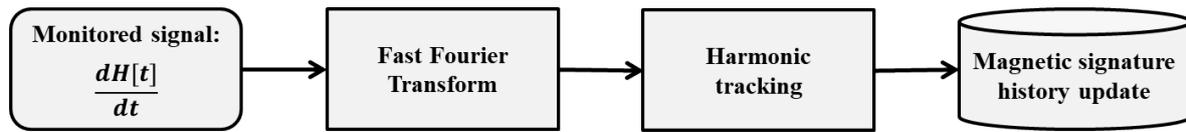
Fig. 3. Data processing for magnetic signature update.
