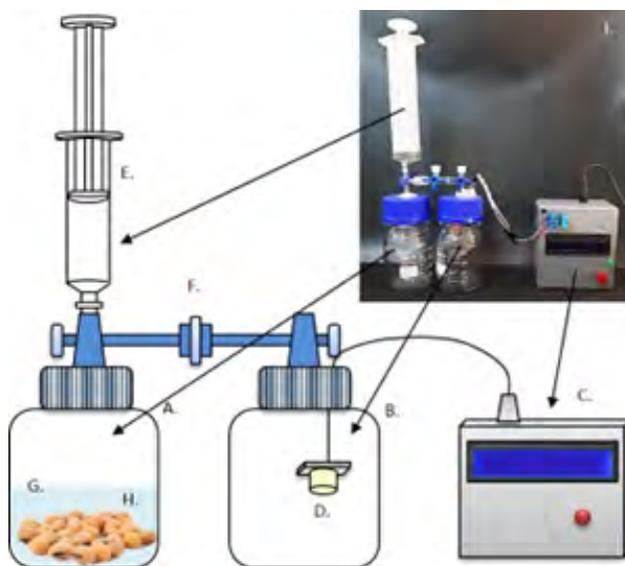
Figure 1. Sketch of the alcohol meter for analysis of soybean seeds. Glass flask A (A), Glass flask B (B), electronic system (C), sensor (D), syringe-type aspirator (E), central valve (F), water (G), soybean seeds (H) and alcohol meter for seed analysis (I).
