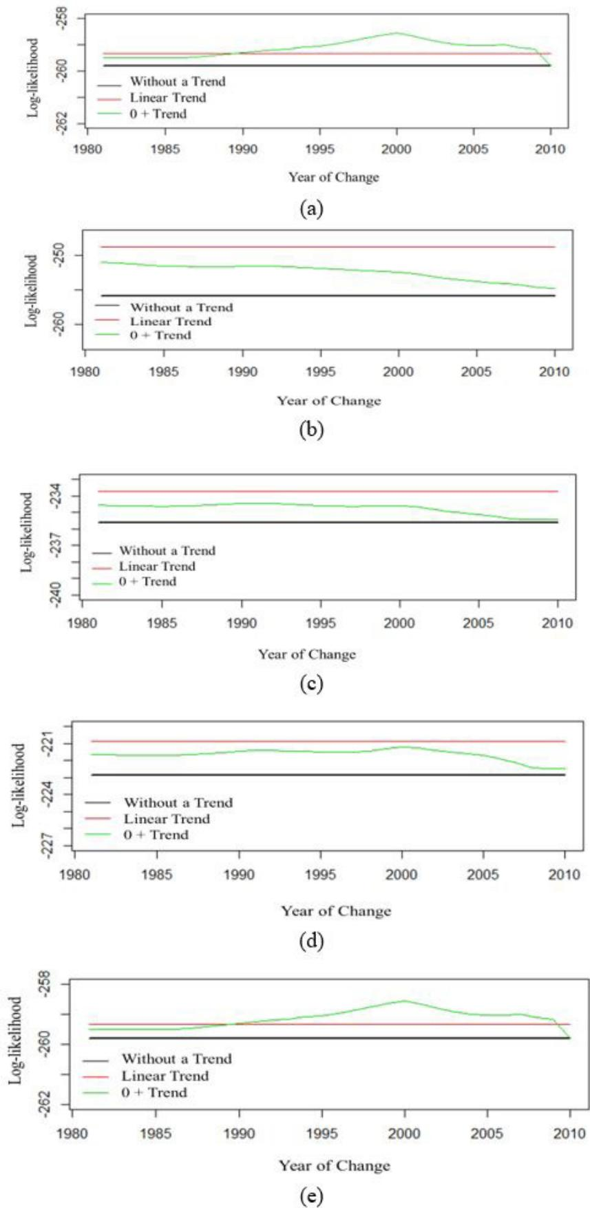
**Figure 4.** Log-likelihood for the three non-stationary models in relation to the year of change for the maximum precipitation series with durations of 10 (a), 15 (b), 30 (c), 45 (d), and 60 (e) min.
