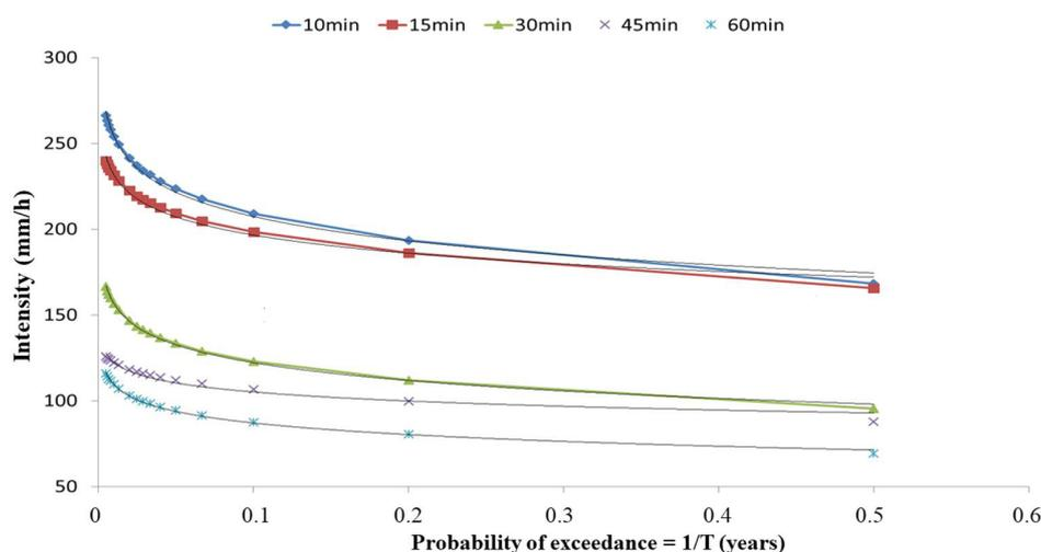
Figure 6. Quantiles of rainfall intensity, in mm/h, for different durations and probabilities of exceedance.
