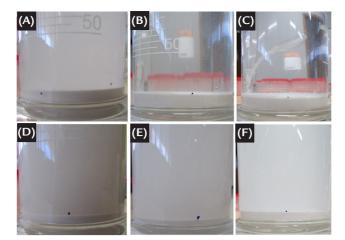
Figure 3 - Final quartz -38+10μm sediment, at 0.2% solids, 550 rpm and at pH 3.0: (A) blank, (B) 300 g/t PAM, (C) 30 g/t PAM, 3.2x10<sup>-5</sup> mol. L<sup>-1</sup> EDA, and at pH 11.0: (D) blank, (E) 300 g/t PAM + EDA 1.6x10<sup>-3</sup> mol. L<sup>-1</sup> EDA, (F) 30 g/t PAM + 3.2x10<sup>-5</sup> mol. L<sup>-1</sup> EDA.
