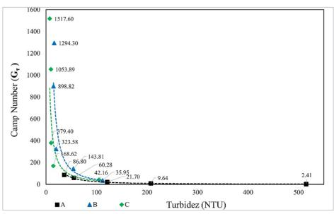
Figure 4 - Camp Number (G $\tau$ ) for the flocculation of quartz sediment -38+10µm, at pH 3.0, 0.2% solids, 3.2x10<sup>-5</sup> mol.L<sup>1</sup> EDA, 550 rpm. (A) blank, (B) 300 g/t PAM, (C) 30 g/t PAM.
