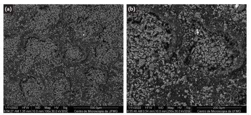
Figure 6 - Backscattered scanning electron microscopy images of flocs formed in condition C. (a) 100x magnification e (b) 250x magnification.
