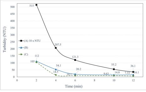
Figure 1 - Turbidity curves of quartz -38+10  $\mu$ m, pH 3.0, 0.2% solids, 3.2x10<sup>-5</sup> mol.L<sup>-1</sup> EDA, 550 rpm. (A) blank (B), 300 g/t PAM, (C) 30 g/t PAM.
