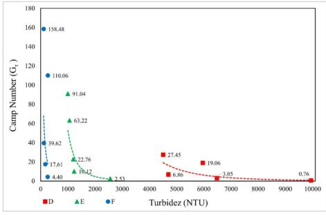
Figure 5 - Camp Number (G $\tau$ ) for the flocculation of quartz sediment -38+10µm, at pH 11.0, 0.2% solids, 550 rpm. (D) blank, (E) 300 g/t PAM + 1.6x10<sup>-3</sup> mol.L<sup>-1</sup> EDA, (F) 30 g/t PAM + 3.2x10<sup>-5</sup> mol.L<sup>-1</sup> EDA.
