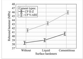
Figure 4 - Effects between the cement type and treatment type on the surface hardness.
