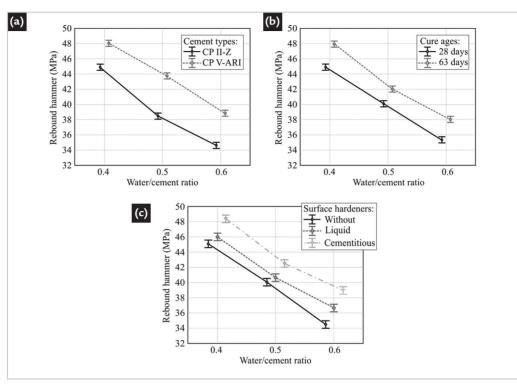
Figure 5 - Effects between the cement type and treatment type on the surface hardness.
