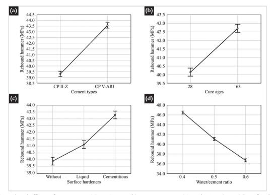
Figure 3 - Isolated effects of cement type (a), curing age (b), treatment type (c), and w/c ratio on (d) surface hardness.
